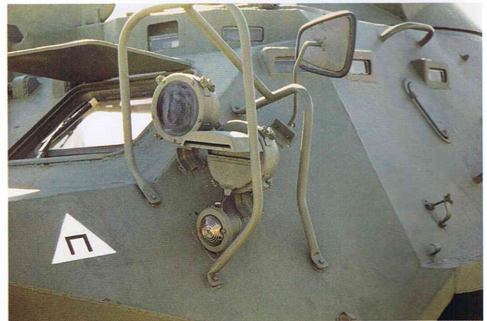
A close-up of the lighting equipment of the BTR-60/TAB-72. Note the shape of the lampguard and the blackout light in the middle.
