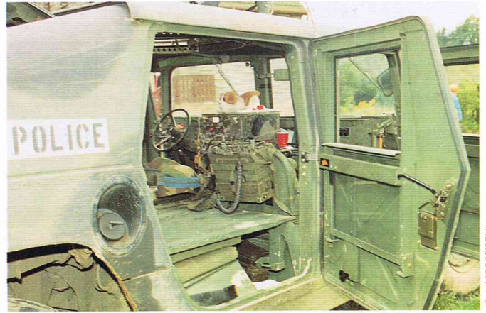
Additional field radios are carried inside this Humvee. This photo clearly shows the installation of the windows and the window raising and lowering mechanism. Here, the Italieri kit leaves a lot to be desired.
