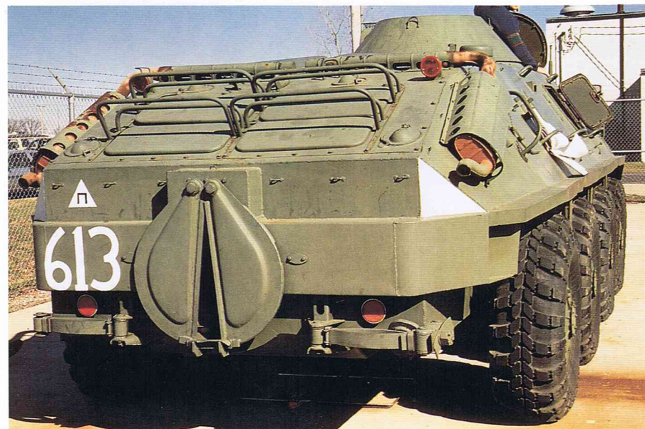
The rear of the vehicle showing the amphibious nature of this design. The split 'kidney-shaped' covers over the controllable propeller outlet can be seen partially opened. The covers on the sloped aft deck open when the hydrojet system is operating.
